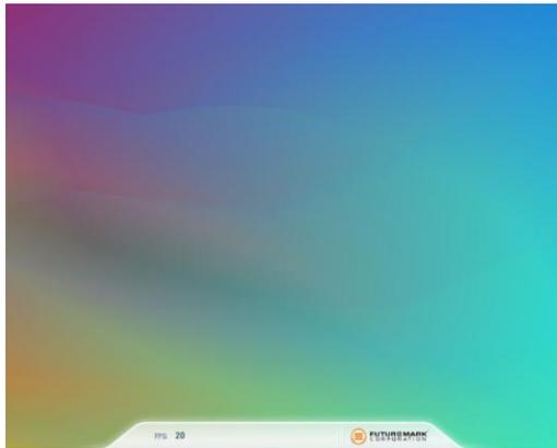
This test draws frames by drawing a rectangle across the screen multiple times. The color and alpha channels of each corner of the rectangle is animated. The pixel shader is pass-through. The interpolated color is written directly to the render target using alpha blending. The render target is in 16-bit floating-point format, currently the most relevant format for HDR rendering output.
