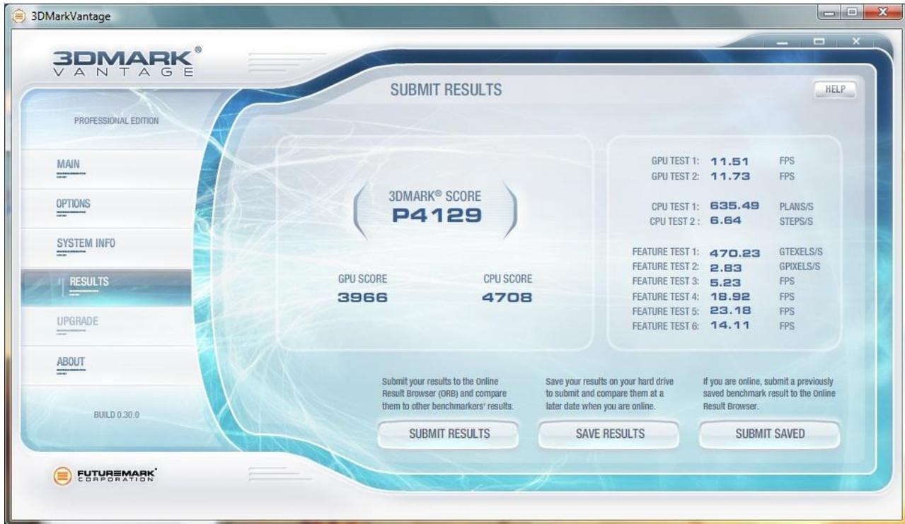
The 3DMark® Score is shown at the top left, prefixed with the letter code for the selected rendering option Preset (P for the Performance Preset in the example). Directly below the main 3DMark® Score are the sub-scores: the GPU Score and the CPU Score. The right side of the results screen is taken up by the raw scores for each test.
